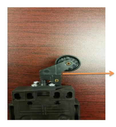
Move part with "jagged teeth" forward. tighten screw back into place.
